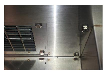
Position the blower box on the outside of the table with the blower mounting bolts (as shown above) so they fit inside the two cut outs on the inside of the table. Then use the four  $\frac{1}{4}$ -20x1/2 bolts and lock washers inside of the bin, through the table wall into the weld nuts inside of the box.
