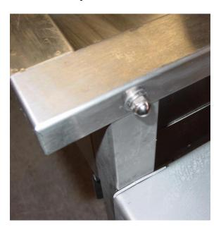
2. Using two 1/2-13 x 2 1/4 BOLTS, two 1/2-13 HEX NUTS, and two 1/2 SPLIT WASHERS, attach the top bolts to hold the SHELF in position, using the topmost holes beneath the SHELF. Insert the BOLTS from the inside of the TRAY, and
